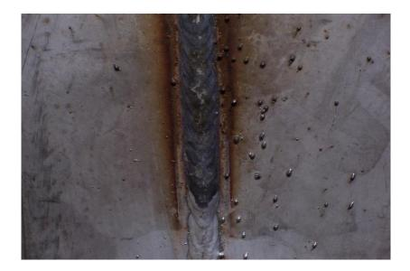
Mechanical removal of the spatter deposits is time consuming and costly, and this re-work can be avoided by the use of special anti spatter sprays. The anti spatter spray leaves a protective oily film on the surface of the steel to prevent spatter from sticking once solidified.
