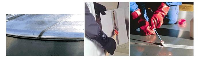
Pickling of stainless steel welds helps to remove both the oxide scale and free iron contamination. Once the pickling agent is completely rinsed away, the treated area will be chemically clean. As such, the surface has an enhanced ability to react with atmospheric oxygen to passivate, providing the area is free from dirt and outside sources of contamination. Newer generation gels are proving to be far more effective and easier to use than older paste based products.
