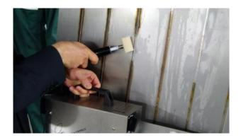
These portable technologies have historically been limited to TIG welding processes where a smooth weld profile will not tear and damage the wand cleaning pads on the tip of the wand.
